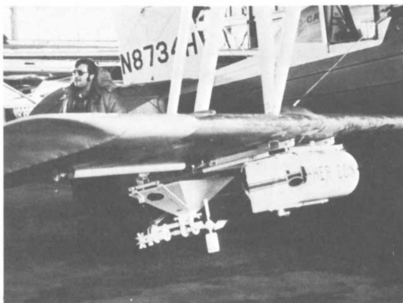
Figure 4. Hercon flake-dispensing equipment used on aircraft.
